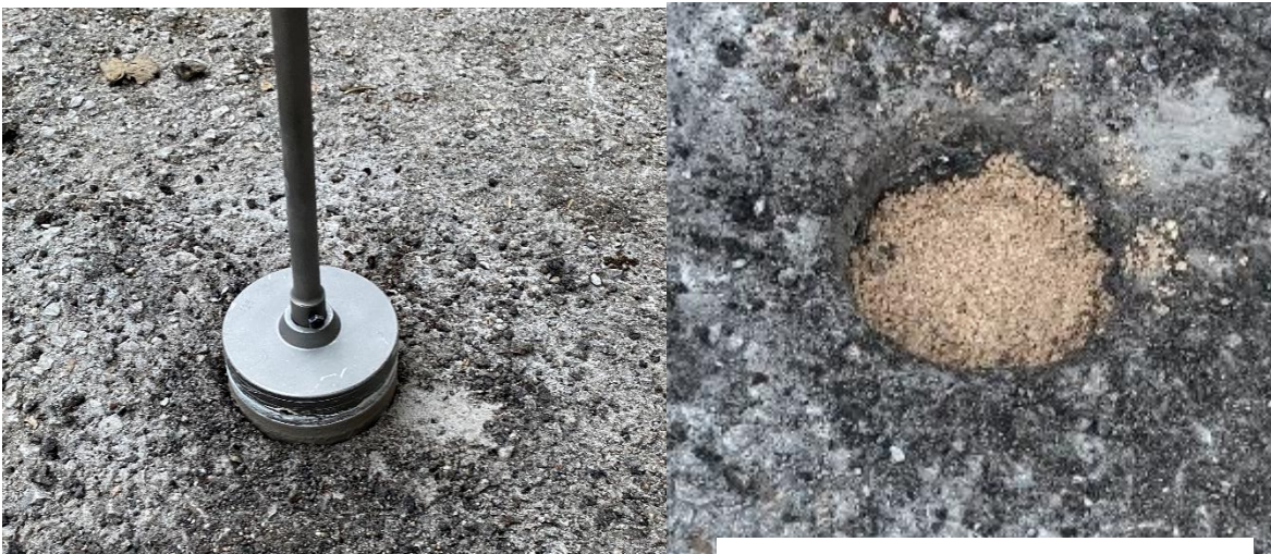
Figure-5: Placing sand in the hole
