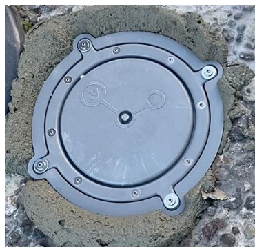
Image: Sensor sitting in the hole, flush to the ground.
